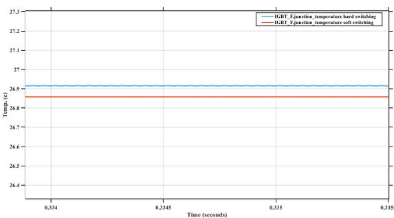
**Fig 5.** Soft and Hard switching junction temperature.
