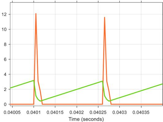
**Fig 3.** Soft switching  $V_{ce}$  and  $I_{ce}$ .
