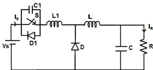
Fig 1. Graphical schematic of the ZVS Buck converter.
